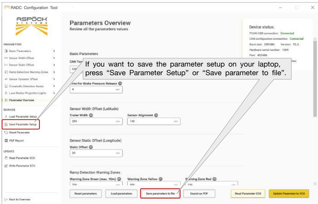
Multiple parameter setups can be stored on the laptop/PC. These can be loaded at any time to adjust them if necessary.
