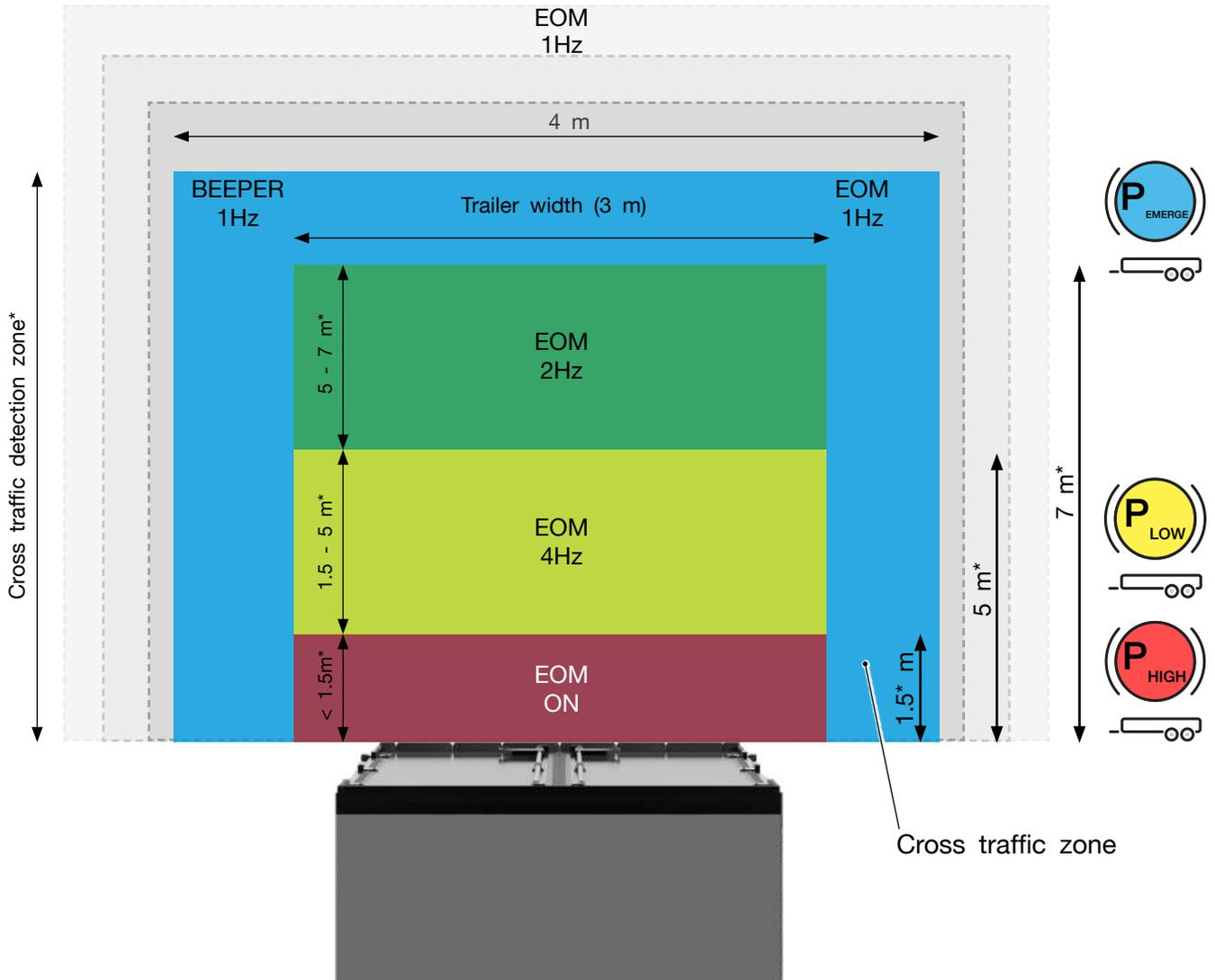
\*Settings can be customized in the RADC 2.0 Configuration Software (9.4).
