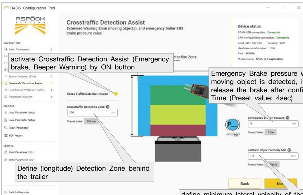
activate Crosstraffic Detection Assist (Emergency brake, Beeper Warning) by ON button
