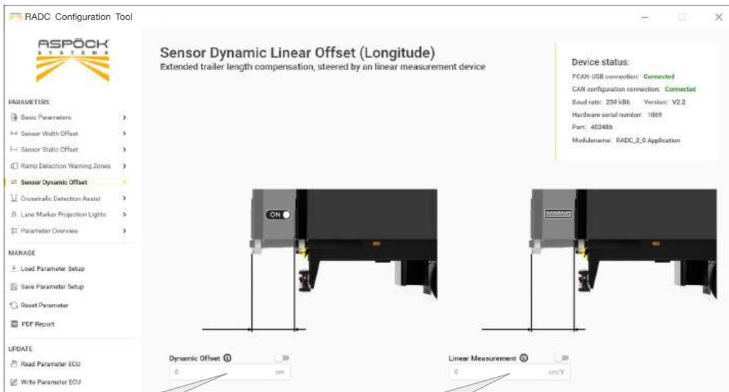
„enter measured distance from Sensor Top surface to last excess length of the trailer.
