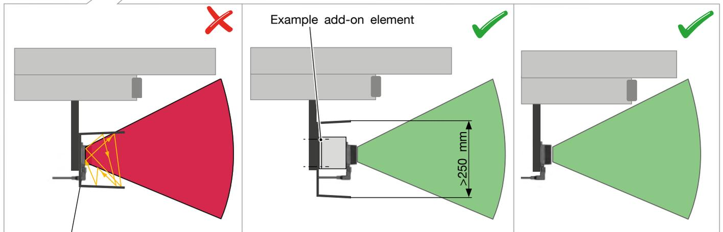
Radar reflections due to excessive depth
