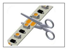
Cut the LED-Stripes at the soldering points
